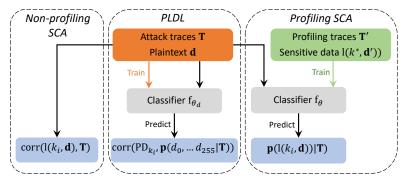
Figure: A demonstration of non-profiling SCA, PLDL, and profiling SCA.
