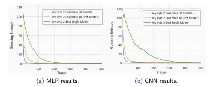
Figure: Guessing entropy for ASCAD for the Hamming weight leakage model.
